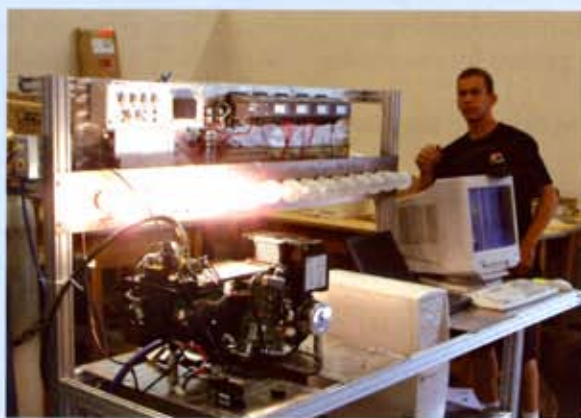
OREC student Ryan Dela tests a 1.2 KW hydrogen-powered fuel cell.
